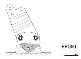
MOTOTRAX SKI BLOCK ORIENTATION MUST BE INSTALLED WITH PLATES P1400222R00 & P1400422R00
