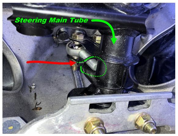
Replace the RH plastic "tie rod guide" with the supplied plug and zip tie.
