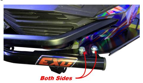
5. Install ANT400 and ANT450 with M8 x 25 Flange Bolts, A-Arms's bolt and A-Arms's washers, without torquing the bolts.
