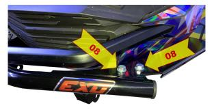
9. Tighten the M8 bolts installed in step #1.
