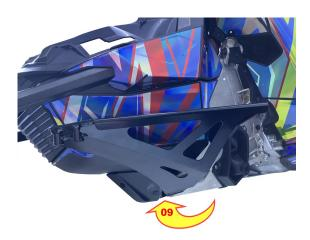
10. Install PNT602S with the stabilizer bar and secure the assembly with the M6 bolt and nut. \* It's normal to have a play between both parts.
