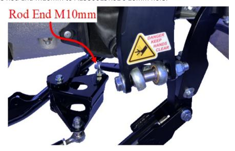
19. Attach the upper portion of the LH shock to ANT400 with the M8 x 55 bolt and nut.
