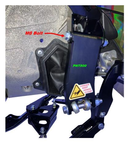
18. Attach the Rod End M10mm to A1530019R01's 10mm hole.
