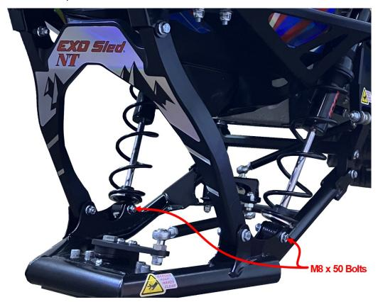
22. Assemble M8 x 70 bolts (3x), PNT142 (2x), PNT141 (2x) and M8 nuts (3x) to PNT140.
