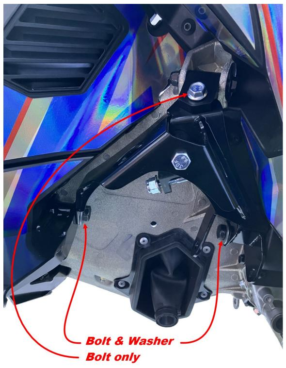
6. Tighten the M8 x 25 Flange bolts installed in step #5.
